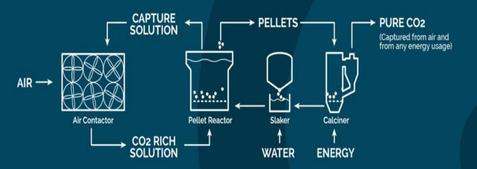
CE's Direct Air Capture process, showing the major unit operations - air contactor, pellet reactor, slaker, and calciner - which collectively capture, purify, and compress atmospheric CO<sub>2</sub>
